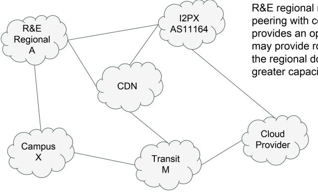
R&E regional network may have local peering with commercial networks that provides an optimal low-latency path. I2PX may provide routes to commercial networks the regional doesn't peer with or that have greater capacity.
