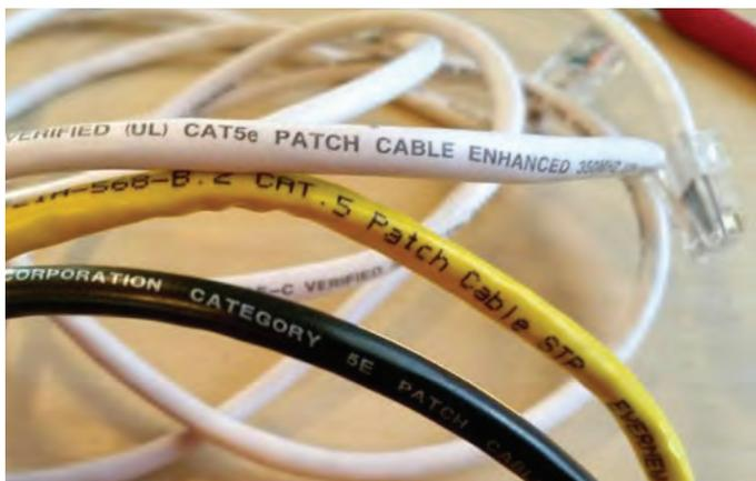
At shorter distances, lower Cat cables can perform at higher speeds, for instance Cat-6 can transfer at 10 Gb/s over lengths up to 55 meters.
