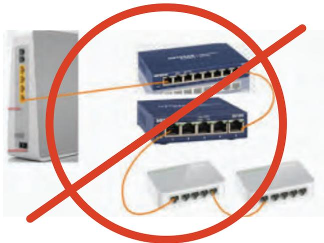
While daisy chaining is a common strategy to create more physical network ports throughout a building, the technique comes with an impact on network performance. The more devices that are daisy-chained the slower the devices on the daisy-chain switches perform. Although some libraries daisy-chain switches together, it is not a best practice in terms of network speed and performance (this article explains more: <https://www.techrepublic.com/blog/it-consultant/only-novices-daisy-chain-switches/>)
